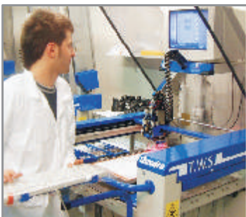
Imbutitura tasti e zone microleds e assemblaggio componenti della tastiera Embossed of the keys and parts and assembling of the keyboard's components
